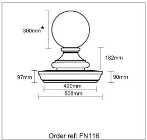
\*NB Ball also available in 230mm and 400mm diameters.
